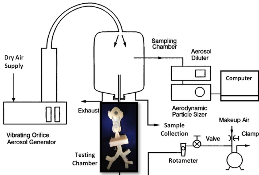
Figure 2. Setup of the Apparatus used for Studying Aerosol Deposition
