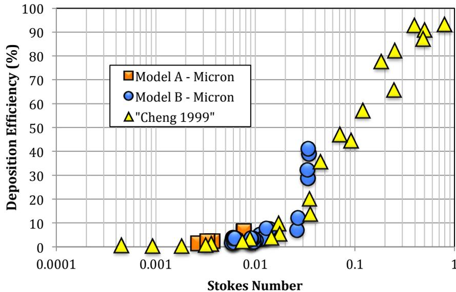
Figure 3. Deposition Fraction vs. Stokes Number
